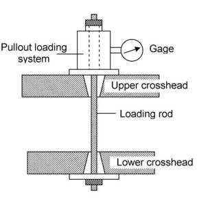
b) Calibration using tension testing machine
