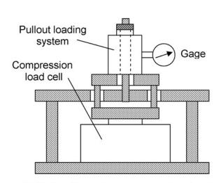
d) Calibration using compression load cell
