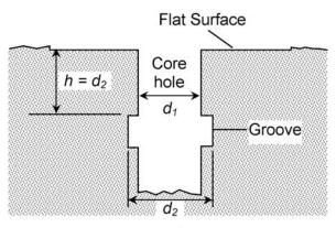
(a) Drill hole, grind surface, and undercut groove
