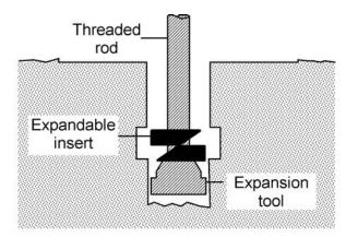
(b) Insert expansion tool and expandable insert
