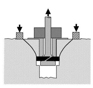
(d) Install bearing ring and loading system; pullout insert assembly
