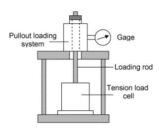
c) Calibration using tension load cell
