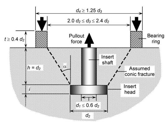
FIG. 1 Schematic Cross Section of Cast-in-Place Pullout Test
