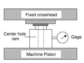
a) Calibration using compression testing machine
