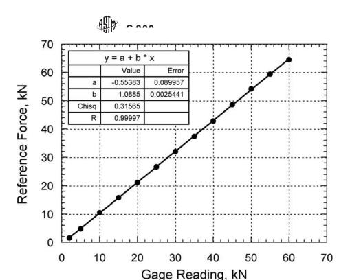
FIG. X2.1 Plot of Calibration Data from Table X2.1 and Best-Fit Straight Line
